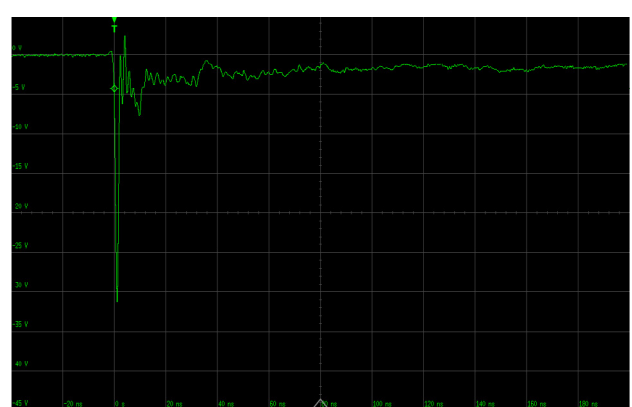
ISO10605 contact discharge plot at -8 kV
