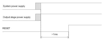
Figure 2-1. Recommended Power Up Sequence
