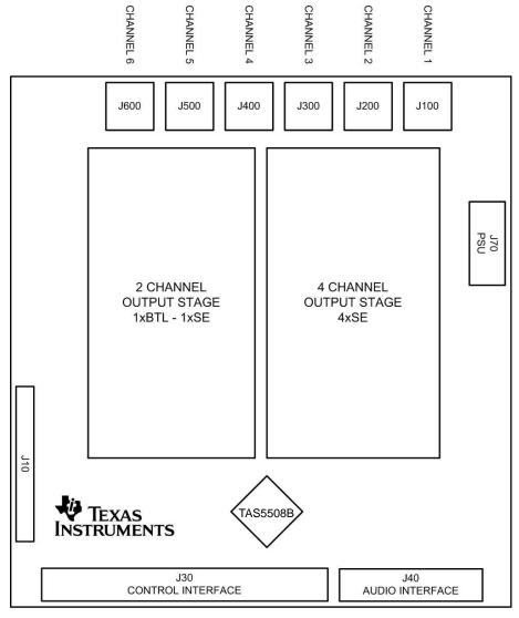
Figure 1-2. Physical Structure for the TAS5508-5122C6EVM (Rough Outline)
