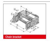
This chain bracket offers universal connection options (top, bottom and front) and is attached to the ends of the chain like a side link. This allows the chain to move right up to the bracket. Each chain requires one male and one female bracket. M5 screws and insert panels are used to secure the brackets in place.
