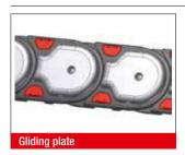
The gliding plates are mounted in a horizontal position, with the chain laying on its side, to minimize friction wear to the sides. They are mounted to the side links using a special screw. The wear limit is 2.5 mm. We recommend replacing the energy chain when this limit has been reached. Depending on the application, the service life of the energy chain may be extended two-fold, by using gliding plates. The energy chain must be placed on its side before opening.
