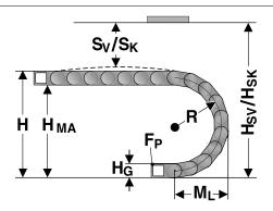
The moving end chain connection is to be screw fixed at height  $H_{\text{M}}$  for the respective radius.
