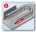
Horizontal installation option, side-mounted (rotated 90°) with support
