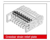
Fixed integrated frame bridge strain relief plates in the chain brackets. Accommodated to all widths of the frame bridges, up to 256 mm in size. May be assembled on the inside and outside flexure curves at both chain endings.
