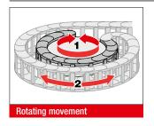
Side links with rearward radius allow movements in both directions. This is intended for rotating movements and lowered chain brackets. Rotation movements are only possible with open variants.
