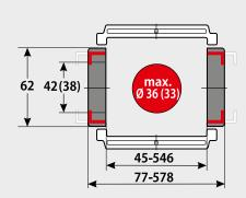
Internal height: 42.0 mm Internal widths: 45.0 - 546.0 mm Radii: 90.0 - 350.0 mm Pitch: 77.0 mm Links per metre: 13 qty. Loading side: Inside and outside bend MP 41.3: inner widths 71-346 mm, radii 150-300 mm, lower inner height (values in brackets)
