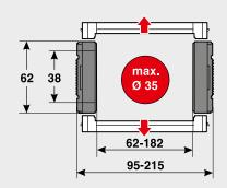
Internal widths: 62.0 - 182.0 mm
