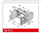
This chain bracket offers universal connection options (top, bottom and front) and is attached to the ends of the chain like a side link. This allows the chain to move right up to the bracket. Each chain requires one male and one female bracket. M10 bolts are used to secure the brackets in place. Metal inserts (supplied) help to minimize the cold flow properties. This is an enormous advantage, guaranteeing the smooth transfer of high loads to the chain.
