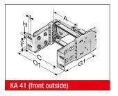
There are several options regarding the chain bracket. The fixed-point bracket (inside/bottom) and the moving end bracket (inside/top) are supplied as standard. However, any other combination can be supplied upon request. The chain bracket is fastened at the end like a side link. This enables the chain to move right up to the bracket. Each chain requires two chain brackets. The brackets should be fastened with M6 screws.
