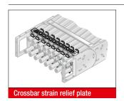
Fixed integrated frame bridge strain relief plates in the chain brackets. Tailored to all crossbar widths up to 200 mm. May be assembled on the inside and outside bends at both chain endings.
