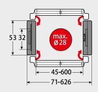
Internal widths: 45.0 – 546.0 mm
