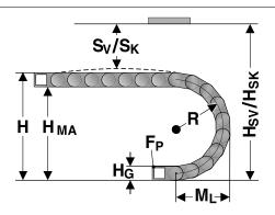
The moving end chain connection is to be screw fixed at height  $H_{\text{MA}}$  for the respective radius.
