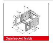
This chain bracket offers universal connection options (top, bottom and front) and is attached to the ends of the chain like a side link. This allows the chain to move right up to the bracket. Each chain requires one male and one female bracket. M8 screws are used to secure the brackets in place. Pressed-in metal bushes with a through-hole ensure the permanent, high-strength transmission of even extreme forces onto the energy chain.
