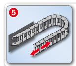
Horizontal installation option, side-mounted (rotated 90°)
