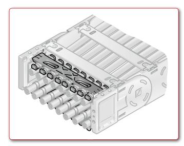
They are secured in much the same way as the crossbars themselves, by snapping them into precut recesses in the chain brackets. This enables two strain relief plates to be integrated into the cable drag chain per cable end, both for the inside bend and the outside bend.
