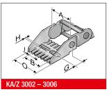
The type KA/Z 3001 - 3006 chain bracket is a plastic part with an extrusion-coated metal insert. The bracket is precisely adjusted to the respective chain width and only needs to be snapped in at the chain link. Please order one male and one female end bracket for each chain. The brackets should be fastened with M6 screws. The cables or tubes may be fastened with cable ties at the integrated strain relief of the chain bracket.
