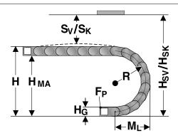
The moving end chain connection is to be screw fixed at height  $\mathbf{H}_{\mathrm{MA}}$  for the respective radius.
