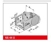
The chain bracket is an all-plastic part. The bracket is precisely adjusted to the respective chain width and only needs to be snapped in at the chain link. Please order one male and one female end bracket for each chain. The brackets should be fastened with M5 screws. The cables or conduits may be fastened with cable ties on the integrated strain relief of the chain bracket.
