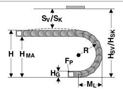
The moving end chain connection is to be screw fixed at height  $H_{\mbox{\tiny MA}}$  for the respective radius.
