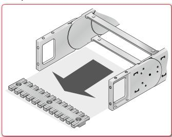
To increase the distance from the strain relief to the first movable point, the strain relief can be moved to a position outside the chain bracket. To do so, you can utilise our Steel Fix bow clamps and ZL-C strain relief plates, which are mounted on C-rails. The ZL strain relief plates can also be secured to a load-bearing substrate directly, without using C-rails.
