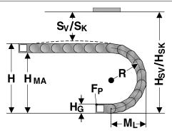
The moving end chain connection is to be screw fixed at height  $H_{\mbox{\tiny MA}}$  for the respective radius.
