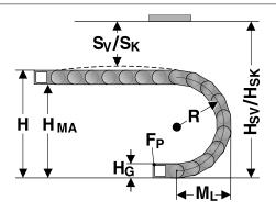
The moving end chain connection is to be screw fixed at height  $H_{MA}$  for the respective radius.
