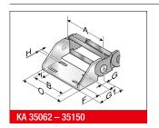
The metal connection (U-section) is precisely adjusted to the respective chain width. It only needs to be snapped in the chain link. Please order one male and one female end bracket for each chain. The brackets should be fastened with M6 screws.
