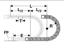
The fixed point of the energy chain should be connected in the middle of the travel distance.
