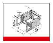
This chain bracket offers universal connection options (top, bottom and front) and is attached to the ends of the chain like a side link. This allows the chain to move right up to the bracket. Each chain requires one male and one female bracket. M8 screws are used to secure the brackets in place. Extrusion-coated metal bushes with either a through-hole (-FB) or a threaded hole (-FG) ensure the permanent, high-strength transmission of even extreme forces onto the energy chain.
