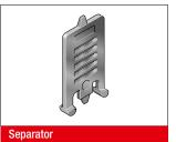
We recommend that separators be used if multiple round cables or conduits with differing diameters are to be installed. The closed separator is used when no shelves are used. This is the recommended design for travel paths of 30 metres or greater.
