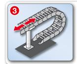
Horizontal installation option, self-supporting, overlap with support
