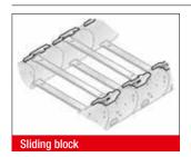
In the case of energy chains, sliding blocks are used in a horizontally sliding installation mode (the tight side of the chain slides on the slack side). The sliding blocks are set onto the side links on the interior bend instead of the usual crossbar interlocks; (no tools needed). This forces the chain to slide on the sliding blocks instead on the side links of the chain. Depending on the application, the service life of the energy chain may be extended five-fold, by using slide blocks.
