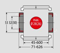
Internal height: 32.0 mm Internal widths: 45.0 - 546.0 mm Radii: 80.0 - 250.0 mm Pitch: 64.5 mm Links per metre: 16 qty. Loading side: Inside and outside bend MP 32.3: inner widths 62-346 mm, radii 120-250 mm, lower inner height (values in brackets)
