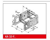
This chain bracket offers universal connection options (top, bottom and front) and is attached to the ends of the chain like a side link. This allows the chain to move right up to the bracket. Each chain requires one male and one female bracket. M5 bolts are used to secure the brackets in place. Extrusion-coated metal bushes with either a through-hole (-FB) or a threaded hole (-FG) ensure the permanent, high-strength transmission of even extreme forces onto the energy chain.
