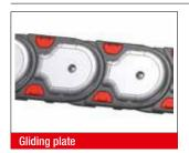
The gliding plates are mounted in a horizontal position, with the chain laying on its side, to minimize friction wear to the sides. They are mounted to the side links using a special screw. The wear limit is 2.5 mm. We recommend replacing the energy chain when this limit has been reached. Depending on the application, the service life of the energy chain may be extended two-fold, by using gliding plates. The energy chain must be placed on its side before opening.
