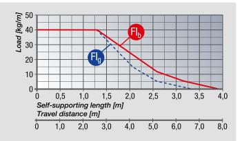
Travel distance gliding L<sub>a</sub> max.: 150.0 m Travel distance vertical, hanging L<sub>vh</sub> max.: 80.0 m Travel distance vertical, upright L<sub>vs</sub> max.: 6.0 m Rotated 90°, unsupported  $L_{90f}$  max.: 1.5 m Speed, gliding V<sub>a</sub> max.: 6.0 m/s Acceleration, gliding a max.: 10.0 m/s<sup>2</sup>
