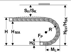
The moving end chain connection is to be screw fixed at height  $\mathbf{H}_{\text{\tiny MA}}$  for the respective radius.
