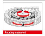
Side links with rearward radius allow movements in both directions. This is intended for rotating movements and lowered chain brackets. Note: This type of chain has different chain links for the left or right side! Rotation movements are only possible with open variants.
