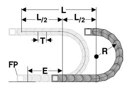
The fixed point of the energy chain should be connected in the middle of the travel distance.
