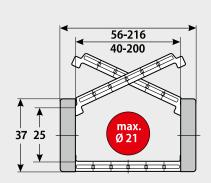
Internal widths: 40.0 - 200.0 mm
