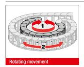
Side links with rearward radius allow movements in both directions. This is intended for rotating movements and lowered chain brackets. Note: This type of chain has different chain links for the left or right side! Rotation movements are only possible with open variants.
