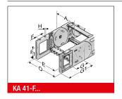
This chain bracket offers universal connection options (top, bottom and front) and is attached to the ends of the chain like a side link. This allows the chain to move right up to the bracket. Each chain requires one male and one female bracket. M6 bolts are used to secure the brackets in place. Extrusion-coated metal bushes with either a through-hole (-FB) or a threaded hole (-FG) ensure the permanent, high-strength transmission of even extreme forces onto the energy chain.
