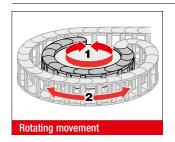
Side links with rearward radius allow movements in both directions. This is intended for rotating movements and lowered chain brackets. The appropriate number of washer discs have to be placed into the side links to achieve the rearward radius.
