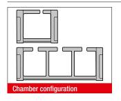
Depending on chain width, the MP10.1 is fitted with one, two, three or four chambers. This system of chambers enables cabling to be laid separately.
