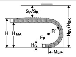
The moving end chain connection is to be screw fixed at height  $\mathbf{H}_{\text{\tiny MA}}$  for the respective radius.
