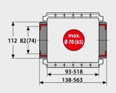
Internal height: 82.0 mm Internal widths: 93.0 - 518.0 mm Radii: 150.0 - 650.0 mm Pitch: 118.0 mm Links per metre: 9 qty. Loading side: Inside and outside bend MP 82.3: inner widths 118-418 mm, radii 200-650 mm, lower inner height
