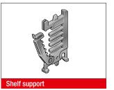
In connection with two separable shelf supports (RTT) with at least one end-to-end shelf (RB) the shelf becomes an easy to fill shelving system. The additional levels prevent cables from criss-crossing and minimise the friction between them.
