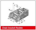
This chain bracket offers universal connection options (top, bottom and front) and is attached to the ends of the energy chain like a side link. This allows the chain to move right up to the bracket. Each energy chain requires one male and one female bracket. M5 screws are used to secure the brackets in place. Press-in metal bushes with a through-hole ensure the permanent, high-strength transmission of even extreme forces onto the energy chain.
