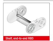
The shelf RBD creates a horizontal separation over the entire width of the chain link. When used together with the TRT 30 separator, an additional, vertical division can be realised.
