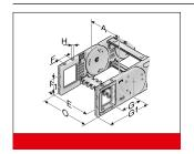
This chain bracket offers universal connection options (top, bottom and front) and is attached to the ends of the chain like a side link. This allows the chain to move right up to the bracket. Each chain requires one male and one female bracket. M8 screws are used to secure the brackets in place. Extrusion-coated metal bushes with either a through-hole (-FB) or a threaded hole (-FG) ensure the permanent, high-strength transmission of even extreme forces onto the energy chain.
