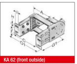
This chain bracket offers universal connection options (top, bottom and front) and is attached to the ends of the chain like a side link. This allows the chain to move right up to the bracket. Each chain requires one male and one female bracket. M8
