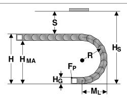
The moving end chain connection is to be screw fixed at height  $\rm H_{MA}$  for the respective radius. For the installed dimension the "Installed height  $\rm H_{S}$  " value has
