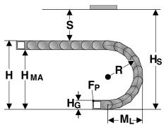
The moving end chain connection is to be screw fixed at height  $H_{\text{MA}}$  for the respective radius. For the installed dimension the "Installed height  $H_{\text{S}}$ " value has to be taken into account.
