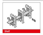
In connection with at least two separable shelf supports (RTT), the shelf becomes a shelving system. The additional levels prevent cables from criss-crossing and minimise the friction between them.
