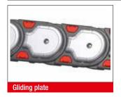
The gliding plates are mounted in a horizontal position, with the chain laying on its side, to minimize friction wear to the sides. They are mounted to the side links using a special screw. The wear limit is 2.5 mm. We recommend replacing the energy chain when this limit has been reached. Depending on the application, the service life of the energy chain may be extended two-fold, by using gliding plates. The energy chain must be placed on its side before opening.
