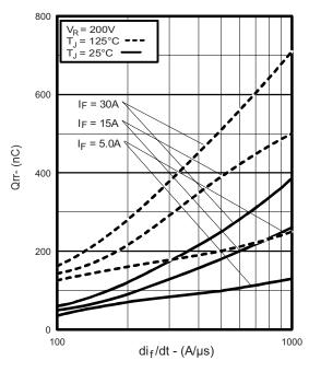
Fig. 7 - Typical Stored Charge vs. dl<sub>F</sub>/dt (Per Leg)
