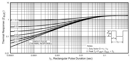
Fig. 4 - Maximum Thermal Impedance Z<sub>thJC</sub> Characteristics (Per Leg)
