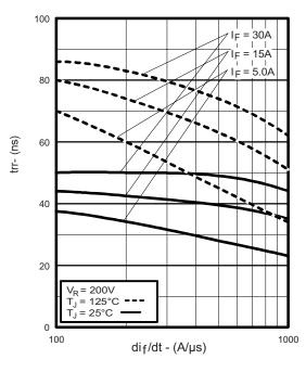
Fig. 5 - Typical Reverse Recovery Time vs. dl<sub>F</sub>/dt (Per Leg)
