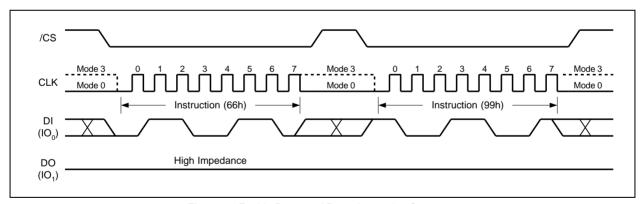
Figure 10. Enable Reset and Reset Instruction Sequence
