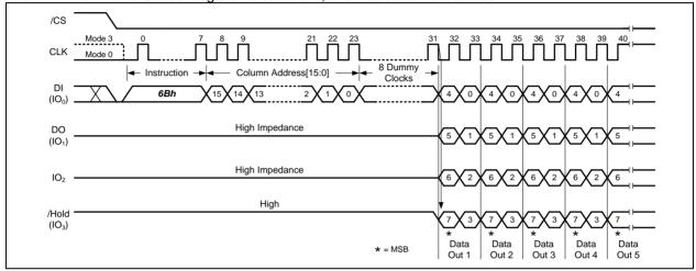
Figure 25. Fast Read Quad Output Instruction
