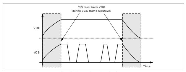
Figure 29. Power-up, Power-Down Requirement
