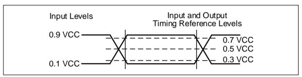
Figure 30. AC Measurement I/O Waveform
