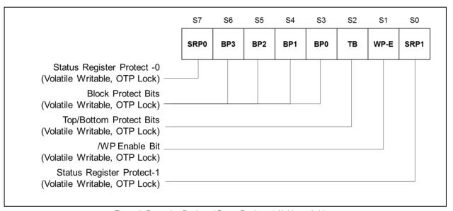
Figure 5. Protection Register / Status Register-1 (Address Axh)
