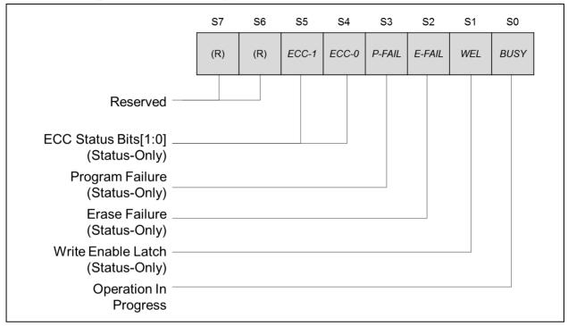
Figure 7. Status Register-3 (Address Cxh)
