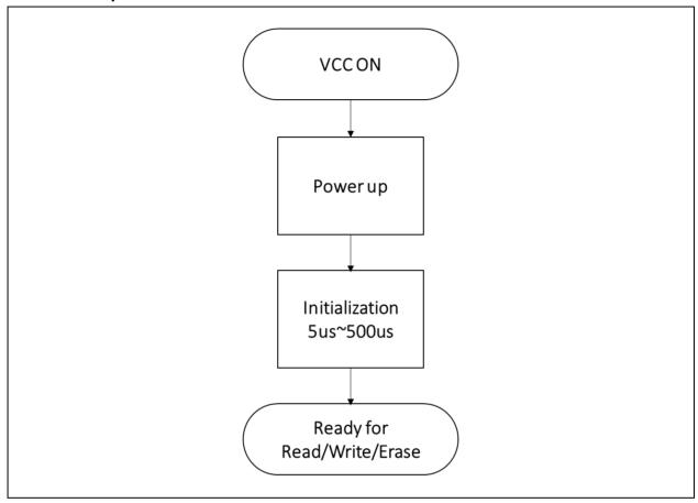
Figure 3. W25N01KV Flash Memory Operation Diagram
