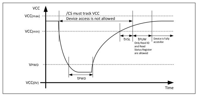
Figure 28. Power-up Timing and Voltage Levels
