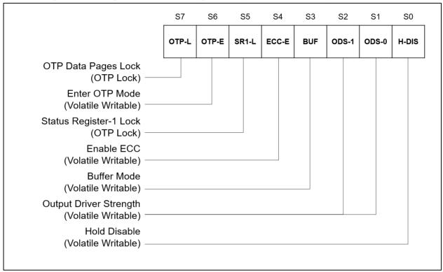
Figure 6. Configuration Register / Status Register-2 (Address Bxh)
