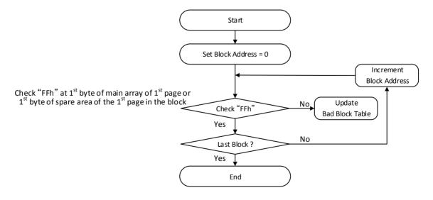
Figure 31. Flow Chart of Create Initial Invalid Block Table
