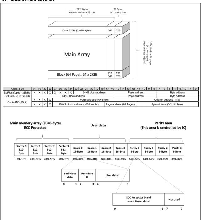
Figure 2. W25N01KV Flash Memory Architecture and Addressing
