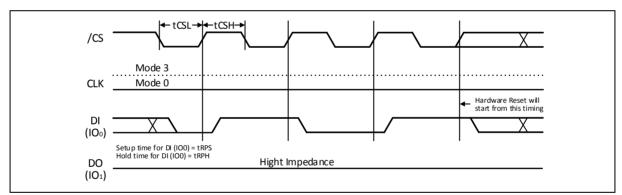
Figure 4. Reset Signaling Protocol
