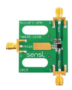
below lists the SMA board connections. The SMA board electrical schematics are available to download in the TSV Board Reference Design document.
