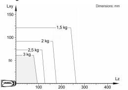
The KR 3 R540 is designed for a rated payload of 2 kg in order to optimize the dynamic performance of the robot. With reduced load center distances, higher loads up to the maximum payload may be used. The specific load case must be verified using KUKA.Load. For further consultation, please contact KUKA Support.
