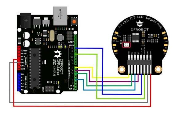
Note: the brightness of the screen can be adjusted through the potentiometer( in the red box of the above diagram). Counterclockwise rotation to brighten the screen.
