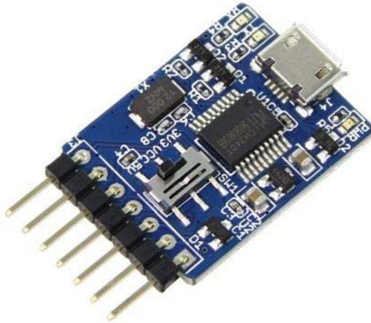
USB To Uart 5V/3V3 is a USB to serial adapter, which is based on CH340. CH340 is a USB bus convert chip and it can realize USB convert to serial interface, USB convert to IrDA infrared or USB convert to printer interface. This module is compatible with 5V and 3V3, and it can be used for uploading code or communicating with MCUs.
