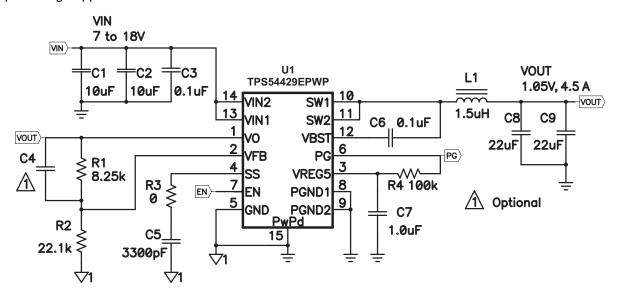
Figure 14. Schematic Diagram for This Design Example
