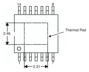
Figure 15. Thermal Pad Dimensions
