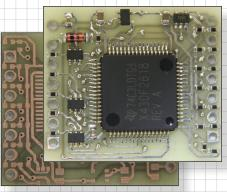
To achieve super-fine traces you must have fast etch times to eliminate under-cutting. By using 1/2oz copper (vs. conventional 1oz) coupled with an .032" fiberglass base, you
