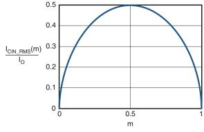
Figure 2. I<sub>CIN</sub> vs. Voltage Conversion Ratio
