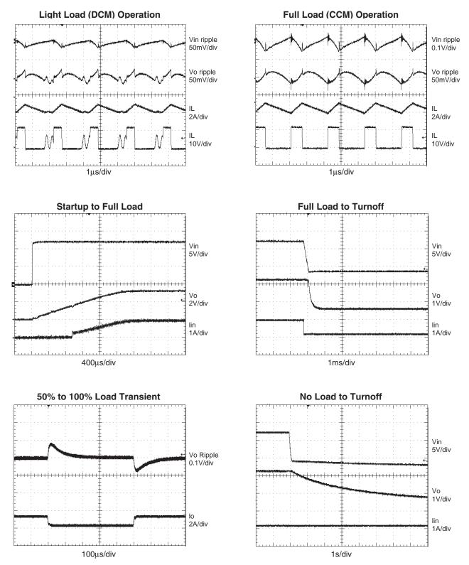
**Typical Performance Characteristics** *(Continued)* Circuit of Figure 1.  $T_A = 25^{\circ}C$ ,  $V_{IN} = V_{EN} = 12V$ ,  $V_{OUT} = 3.3V$  unless otherwise specified.
