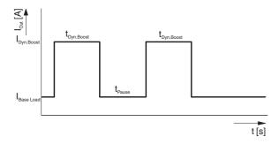
Figure 16 Basic curve of the dynamic boost process
