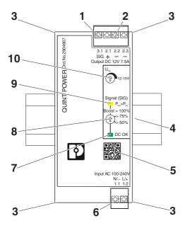
Figure 2 Operating and indication elements
