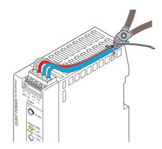
Figure 11 Shorten protruding ends of the cable binder
