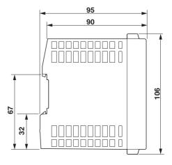
Figure 4 Device dimensions (dimensions in mm)
