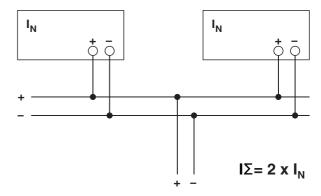
Figure 26 Schematic diagram of increased performance
