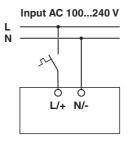
Figure 13 Pin assignment for AC supply voltage
