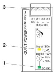
Figure 19 Position of signaling elements
