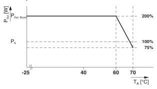
Figure 27 Output power depending on the ambient temperature
