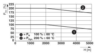
Figure 28 Output power depending on the installation height
