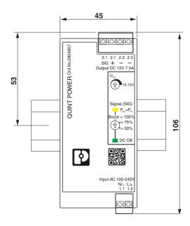
Figure 3 Device dimensions (dimensions in mm)
