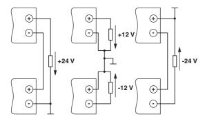
Figure 23 Schematic diagrams in series operation
