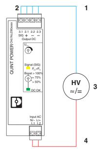
Figure 1 Potential-related wiring for the high-voltage test
