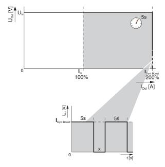
Figure 15 U/I output characteristic curve
