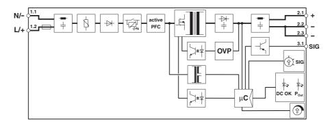
Figure 6 Block diagram
