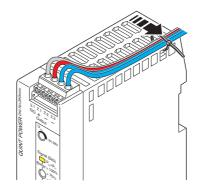
Figure 10 Secure connection wiring with cable binder
