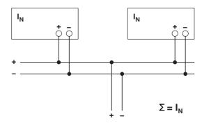
Figure 24 Schematic diagram in parallel operation
