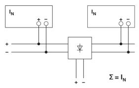
Figure 25 Schematic diagram, redundant operation with diode
