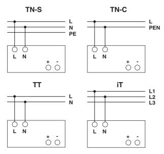
Figure 12 Network configurations in star network
