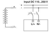
Figure 14 Pin assignment for DC supply voltage
