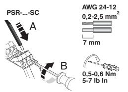
Figure 11 Connecting the cables for PSR-...-SC (screw terminal block)
