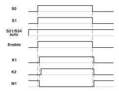
Figure 2 Time diagram for automatic start
