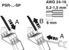
Figure 12 Connecting the cables for PSR-...-SC (spring-cage terminal block)
