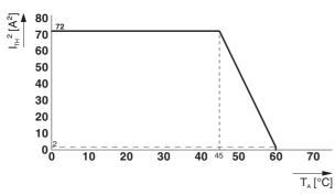
Figure 7 Derating curve
