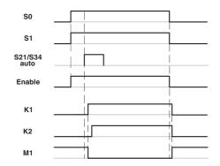
Figure 3 Time diagram for automatic start
