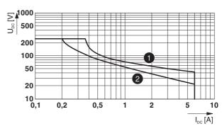
Figure 8 Relay load curve - ohmic and inductive load
