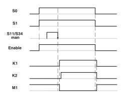
Figure 4 Time diagram for manual, monitored start
