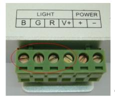
Colour coded screw terminals for LED strip.
