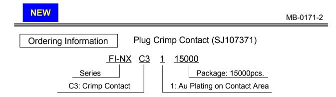
Applicable Wire: 30 to 36 AWG, twisted pair Coated Diameter: 0.45 to 0.50 mm dia.
