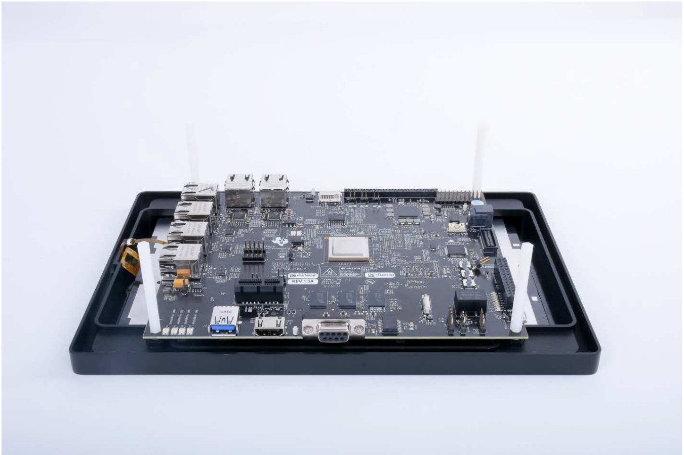
Figure 4. AM574x IDK EVM with LCD Display Assembly Attached - Bottom View
