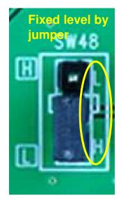
Jumper indicated in the left figure is adopted on this evaluation board to set operation of the TB67S149FTG.
