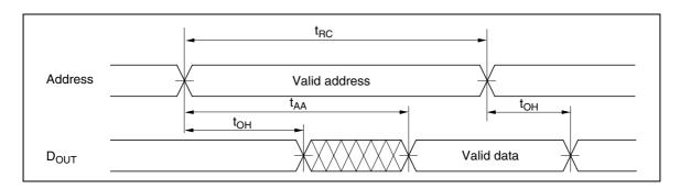
Read Timing Waveform (3) (WE# =  $V_{IH}$ , CS# =  $V_{IL}$ , OE# =  $V_{IL}$ )\* $^2$
