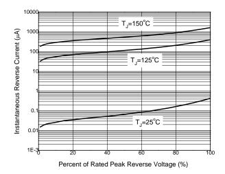
Figure 2. Typical Reverse Current Per Diode
