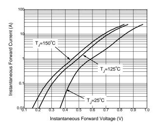
Figure 1. Typical Forward Voltage Per Diode
