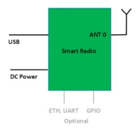
The Mesh Rider Radio has been designed to be plug and play. Only USB and a power supply are required for integration.
