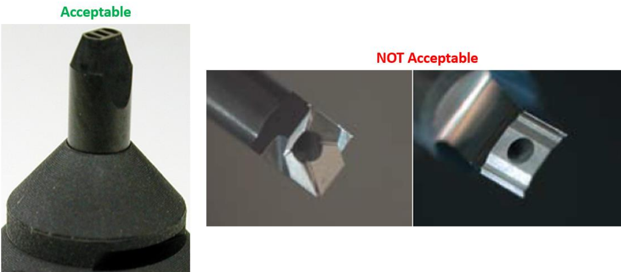
Figure 8: Acceptable vs. NOT Acceptable Tip Shapes
