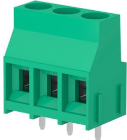
Number of poles: 3, Clamp tightening, 41A, 4mm<sup>2</sup>, 10AWG, 450V, Pitch 6,35 mm, Modular, Connection Angle 0°, Number of levels: 1, Green (RAL 6032), Soldering technology Wave, UL, VDE, IMQ, CSA
