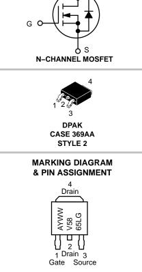
A = Assembly Location\* Y = Year WW = Work Week V5865L = Device Code G = Pb-Free Package
