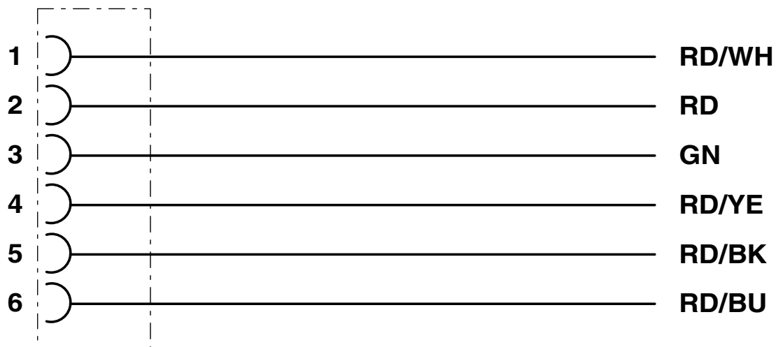
Contact assignment of 1/2" UNF plugs / sockets
