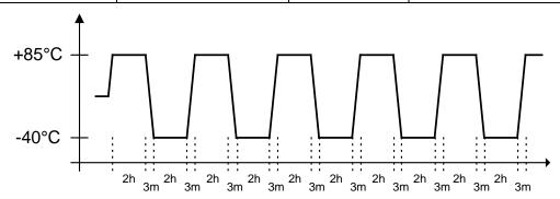
Figure 4-1: Temperature Cycle Test
