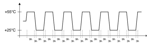
Figure 4-2: Temperature / Relative Humidity Cycle Test
