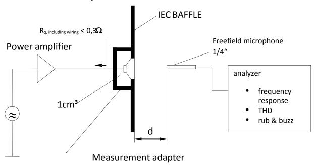
Measurement signal: Logarithmic sine sweep, 1.5s, 22kHz-180Hz
