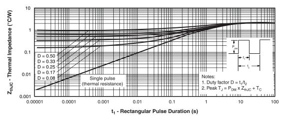
Fig. 4 - Maximum Thermal Impedance  $Z_{\text{thJC}}$  Characteristics
