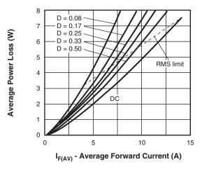
Fig. 6 - Forward Power Loss Characteristics
