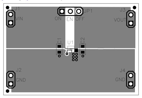
Figure 3. Assembly Layer
