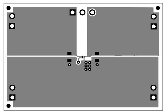
Figure 4. Top Layer Routing
