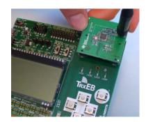
Insert the CC1175EM into a TrxEB. The The TrxEB also makes it easy to control CC1175 connectors will only fit in one position so that the from SmartRF™ Studio and it can be used as a EM cannot be inserted the wrong way. Do not use excessive force on the EM. Remember to mount the antenna.
