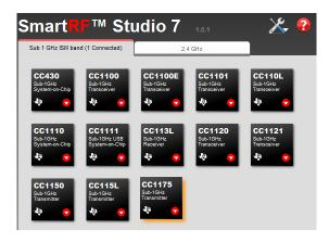
After installing the tool, connect the TrxEB to the PC using the USB cable and start SmartRF Studio. Select the "Sub 1 GHz" tab and double click the highlighted CC1175 device icon.
