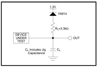
Figure 17. Transient Equivalent Testing
