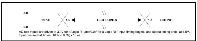
Figure 16. Transient Input/Output Reference Waveform for V<sub>CC</sub>=5V±0.5V (Standard Testing Configuration)
