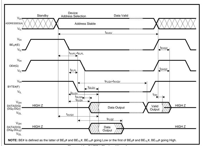
Figure 19. BYTE# Timing Waveforms
