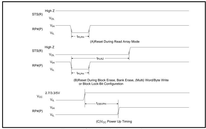
Figure 22. AC Waveform for Reset Operation
