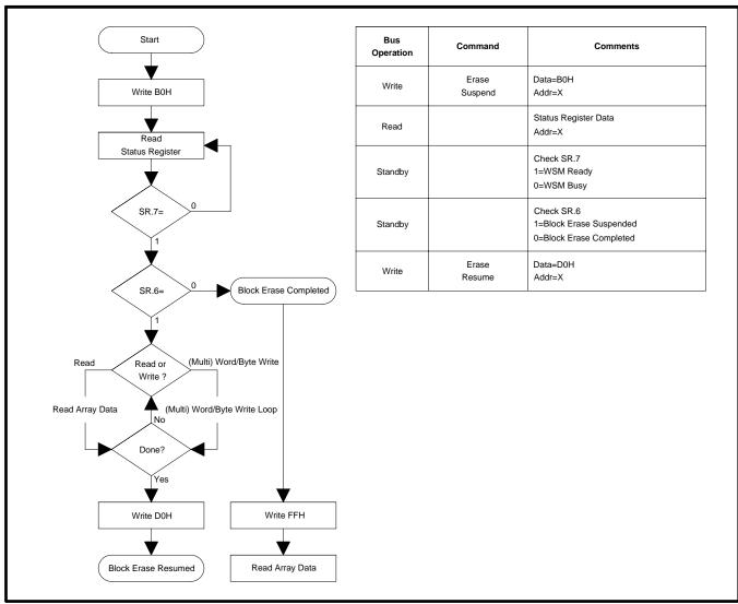
Figure 10. Block Erase Suspend/Resume Flowchart
