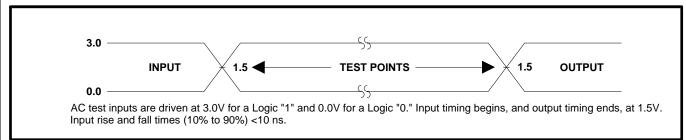
Figure 15. Transient Input/Output Reference Waveform for V<sub>CC</sub>=3.3V±0.3V and V<sub>CC</sub>=5V±0.25V (High Speed Testing Configuration)
