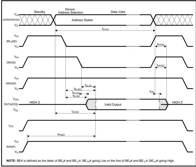
Figure 18. AC Waveform for Read Operations
