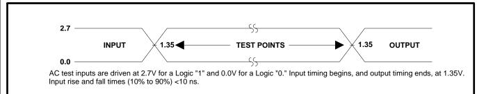
Figure 14. Transient Input/Output Reference Waveform for V<sub>CC</sub>=2.7V-3.6V
