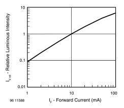
Figure 7. Relative Luminous Intensity vs. Forward Current
