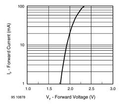
Figure 4. Forward Current vs. Forward Voltage
