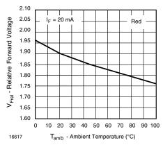
Figure 9. Forward Voltage vs. Ambient Temperature
