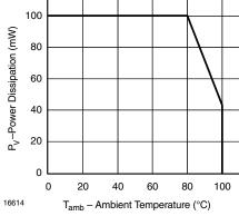
Figure 1. Power Dissipation vs. Ambient Temperature
