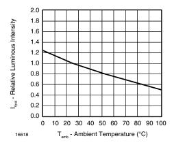
Figure 5. Rel. Luminous Intensity vs. Ambient Temperature
