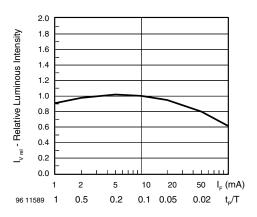
Figure 6. Rel. Lumin. Intensity vs. Forw. Current/Duty Cycle
