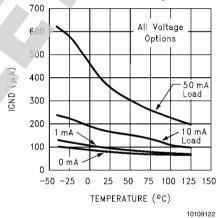
Ground Pin Current vs Load Current
