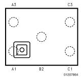
**Note:** The actual physical placement of the package marking will vary from part to part. Package marking contains date code and lot traceability information, and will vary considerably. Package marking does not correlate to device type.
