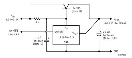
FIGURE 7. 5V to 3.3V @ 3A Converter
