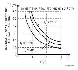
FIGURE 8. Heatsink Thermal Resistance Requirements for Figure 7
