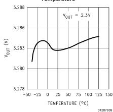
Output Voltage vs Temperature
