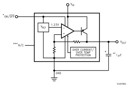
$^{\star}$ ON/ $\overline{\text{OFF}}$  input must be actively terminated. Tie to  $V_{\text{IN}}$  if this function is not to be used.
