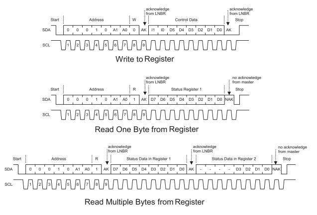
Figure 2. I<sup>2</sup>C<sup>™</sup> Interface. Read and write sequences.
