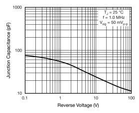
Fig. 5 - Typical Junction Capacitance
