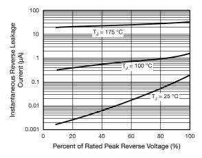
Fig. 4 - Typical Reverse Leakage Characteristics
