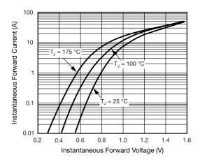
Fig. 3 - Typical Instantaneous Forward Characteristics
