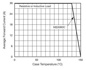
Fig. 1 - Forward Current Derating Curve
