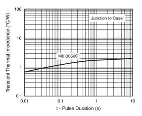
Fig. 6 - Typical Transient Thermal Impedance Per Diode
