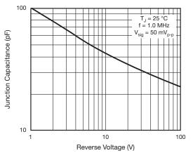
Fig. 5 - Typical Junction Capacitance
