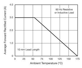
Fig. 1 - Forward Current Derating Curve
