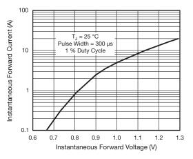
Fig. 4 - Typical Instantaneous Forward Characteristics
