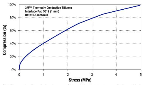
**Note:** Compression vs Stress test results can vary between test methods based on sample size, exact test set-up, equipment type, etc.
