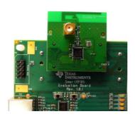
The CC2533EM can be plugged into the SmartRF05EB.
