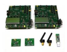
2 x CC2533EM with PCB antennas 2 x 2.4 GHz SMA antennas 2 x SmartRF05EB (prototype boards) 1 x CC2531 USB Dongle (packet sniffer) Batteries, cables and documentation
