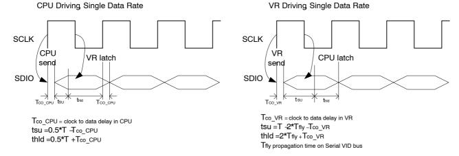
Figure 4. SVID Timing Diagram
