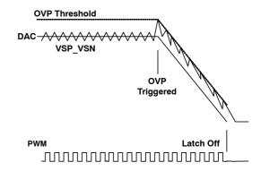
Figure 15. OVP Threshold Behavior
