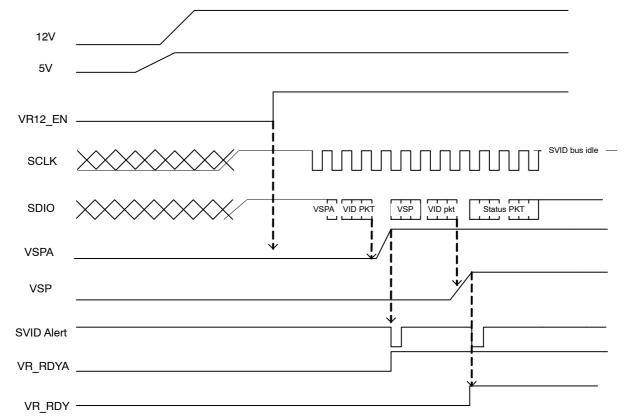
Figure 3. Start-Up Timing Diagram
