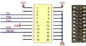
**Note:** depending on the programmer, it is necessary to place pull-up resistors to VCC on the signals RESET, TDI, TMS and TCK. We recommend 100 k ohms.
