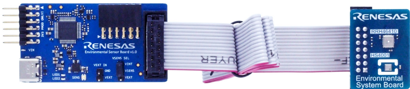
Figure 3. Using a 14-Pin Ribbon Cable to Increase Distance between Communication and Sensor Board
