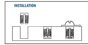
To install, simply press the insert into the hole. The insert compresses as it is installed. As the fastener is threaded into place, the insert expands and the diamond knurling secures it in place.
