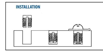
To install, simply press the insert into the hole. The insert compresses as it is installed. As the fastener is threaded into place, the insert expands and the diamond knurling secures it in place.
