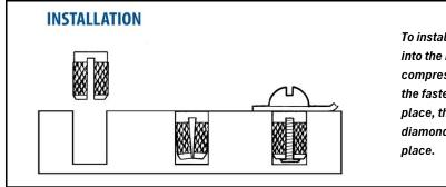
To install, simply press the insert into the hole. The insert compresses as it is installed. As the fastener is threaded into place, the insert expands and the diamond knurling secures it in place.
