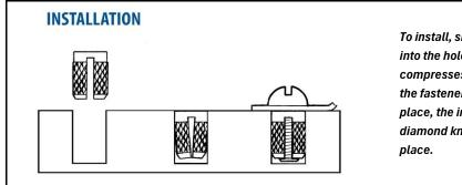
To install, simply press the insert into the hole. The insert compresses as it is installed. As the fastener is threaded into place, the insert expands and the diamond knurling secures it in place.
