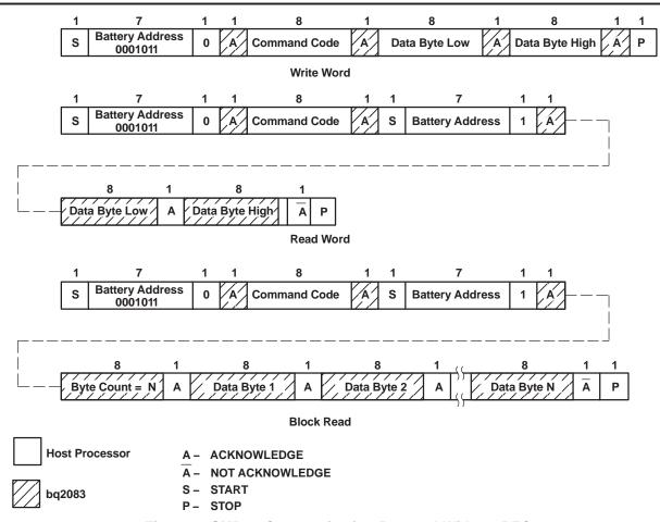
Figure 6. SMBus Communication Protocol Without PEC
