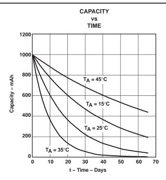
Figure 4. Self-Discharge at 2.5%/Day at 25°C
