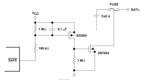
Figure 5. Example SAFE Circuit Implementation
