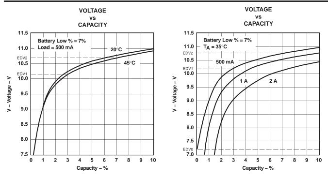
Figure 8. EDV Calculations vs Capacity for Various Temperatures
