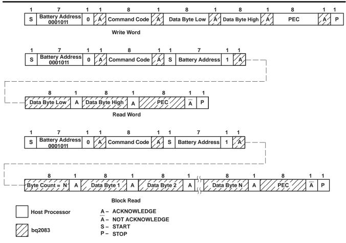
Figure 7. SMBus Communication Protocol With PEC
