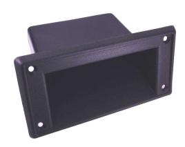
CH-1 is a plastic pocket handle for use on wood or metal enclosures up to 19mm thick. It has 4mm fixing holes.
