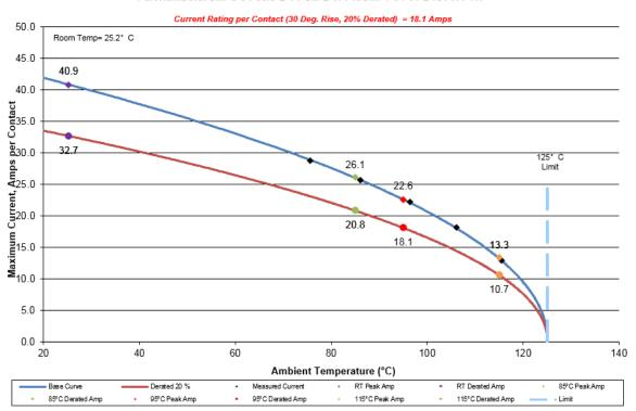
Tracking Code: 2410700\_Report\_Rev\_2 Part #: UMPS-04-05.5-G-V-S-W-TR/ UMPT-04-01-T-RA-WT-TR
