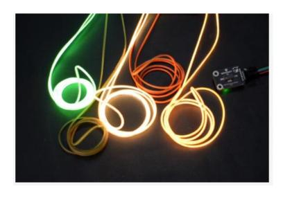
This high-brightness flexible filament has a diameter of only 2mm and a length of 600mm. It is composed of 320 LEDs and can be used for DIY lighting decoration and 360° all-angle lighting fixtures. It requires a power supply of 12V and comes with adjustable brightness. The small round hole end is the positive electrode, and the non-porous end is the negative electrode. The filament can be bent and folded at will, with 360-degree light without dead angles.
